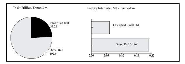
Although Queensland uses electricity as the energy source for bulk (coal) rail, the RTSA does not see this translating to other jurisdictions. In fact NSW retreated from electric locomotive for its coal haulage some decades ago. Diesel locomotives for the haulage of iron ore and coal in WA and NSW continues to be the prime tractive effort.
