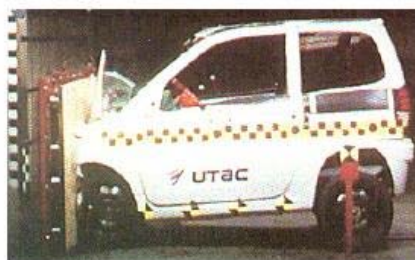
MICROCAR FRONTAL IMPACT TEST
