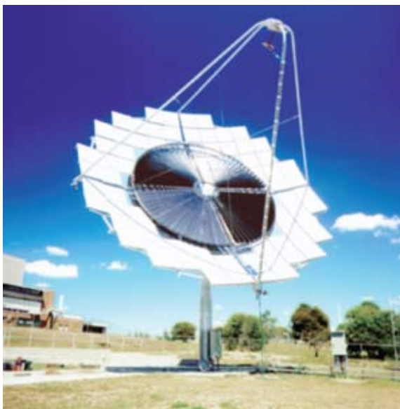
Figure 2.2 CSIRO Solar Collector. Composed of an array of 48 mirrors (area 107m 2 ), on a clear day the array can concentrate 91 kW of thermal energy. © CSIRO
