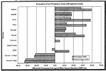
By introducing new processes, which decrease the environmental impact, there can also be a long term cost savings as demonstrated by the HIsmelt process in iron ore production.
