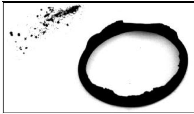
FIGURE 8-1: FORD FALCON SENDER UNIT SEAL - OVER 200,000 KM EXCLUSIVELY ON E10
