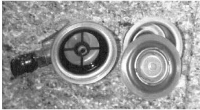
FIGURE 9-1: FUEL PRESSURE REGULATOR SHOWING NO SIGNS OF DETERIORATION
