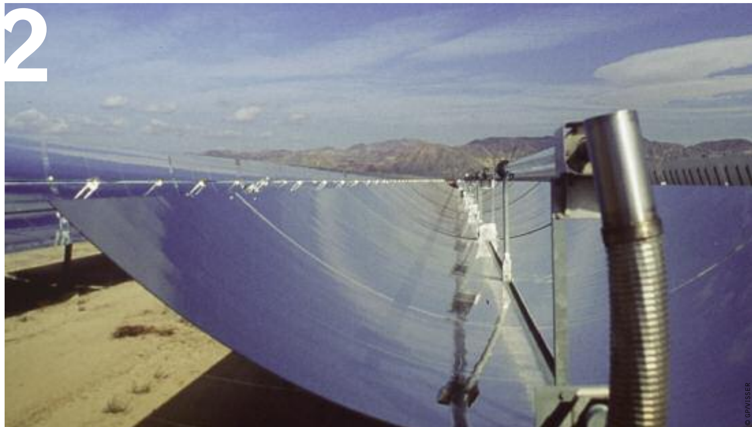
image CONCENTRATING SOLAR POWER (CSP) AT A SOLAR FARM IN DAGGETT, CALIFORNIA, USA.
