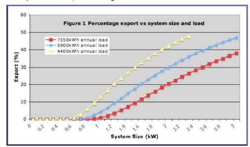
Using average solar insolation data, this can be estimated with a fair degree of accuracy for a FiT based on total generation, but is much more difficult for a FiT based on net export because this is also affected by the household load by time of use, which is more difficult to estimate. For other technologies, such as wind, it would be even more difficult to estimate.
