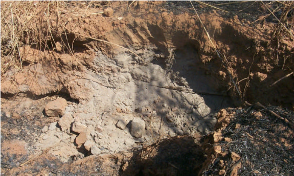
Figure 8. Tailings material removed from an auger hole in the category 4 zone. The surrounding brown/yellow soil can be seen as patches in the black/gray background (which is largely ash from the recent burn off). The undiluted tailings are light gray in colour and comprise all of the material removed from the 1.5 m hole.
