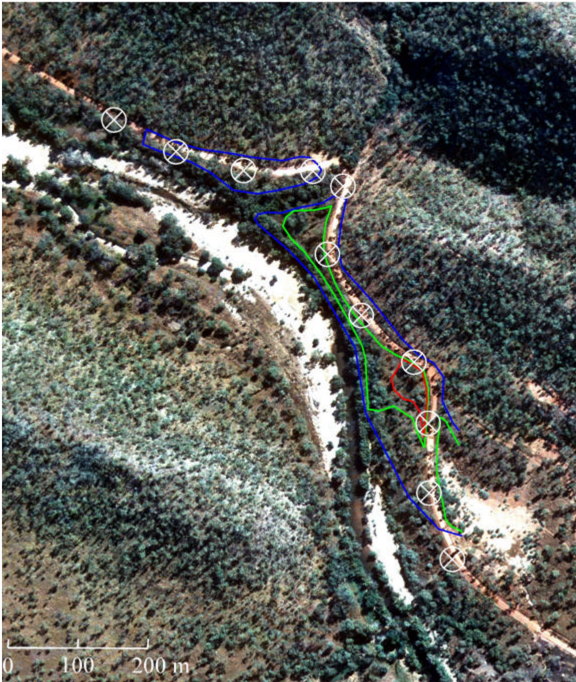
Figure 4. Aerial photograph of the Rockhole mine site area. The sites of the 11 measurements from the 1999 gamma dose-rate survey are indicated. The red, green and blue lines respectively correspond to the approximate extents of the category 4, 3 and 2 areas discussed in the text.
