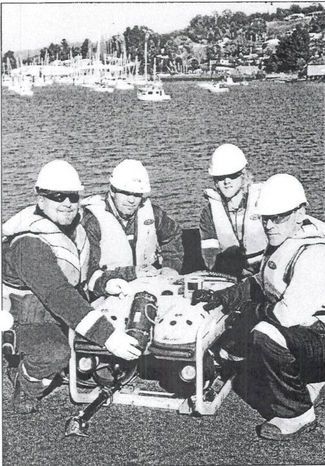
The Underwater Centre head of ROV training Paul Bury and Nicolas Lancelot, of Singapore, Keisey Trelour, of Sheffield, and Joel Parker, of Queensland, look at a Remotely Operated Vehicle, which is an unmanned robotic submersible controlled from the surface. Picture: PAUL SCAMBLER
