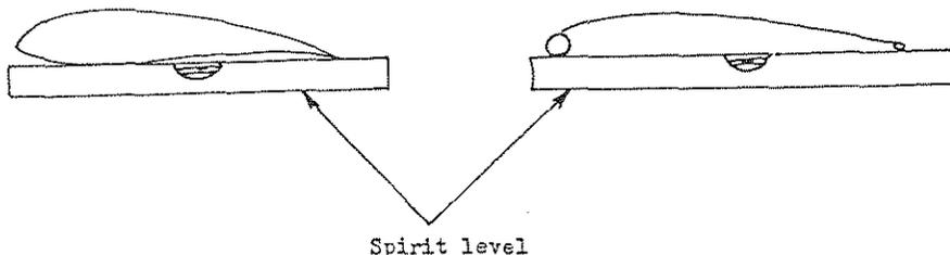
Diagram 1: Method of levelling aircraft by reference to undersurface of wing root aerofoil section.
