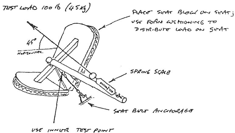
FIG. 1 : SEAT BELT ANCHORAGE TEST
