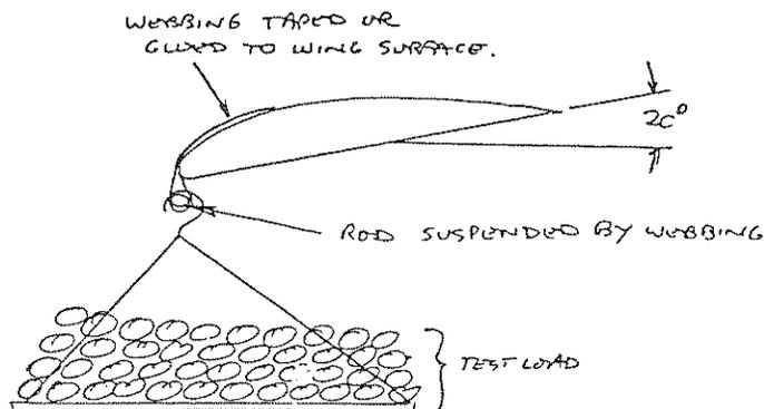
SUPPORT OF AIRCRAFT FOR STRUCTURAL TESTING OF WINGS
