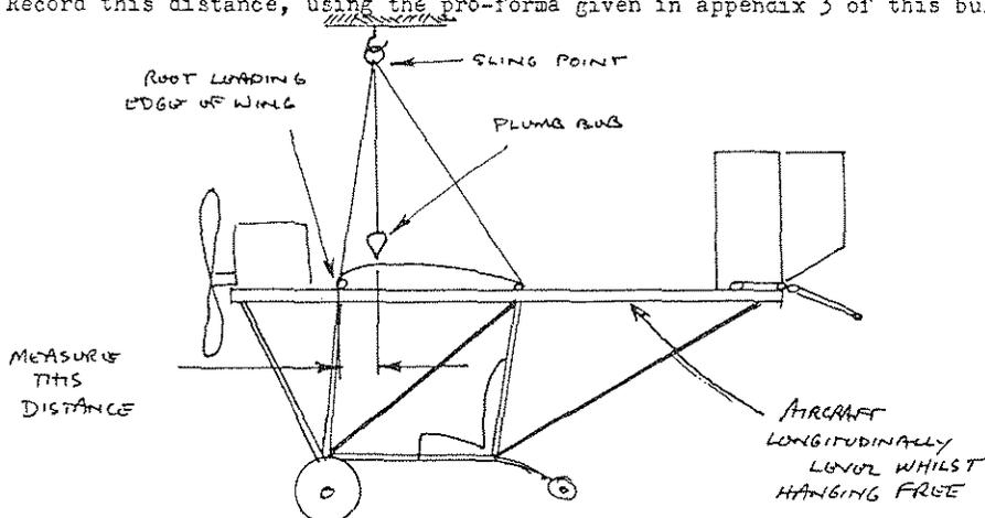
Diagram 2: Use of plumb-bob to determine empty aircraft centre of gravity position.
