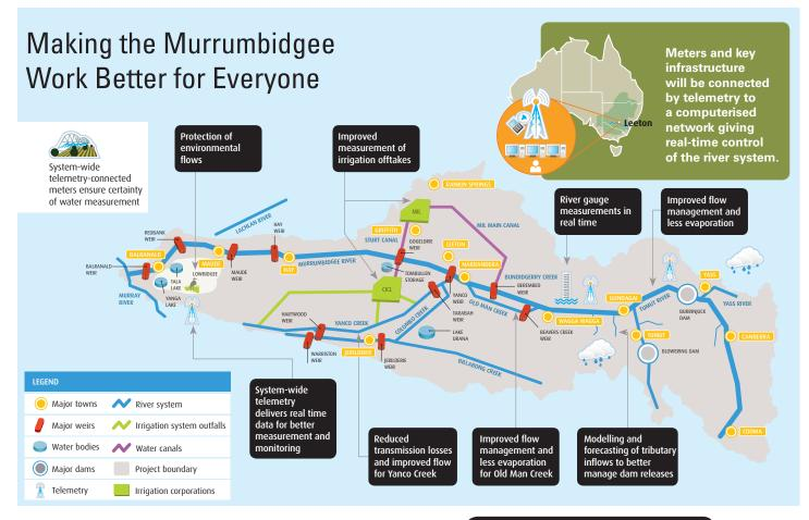
The Murrumbidgee Computer Aided River Management (CARM) project is an upgrade of infrastructure and installation of new interactive river flow management technology throughout the river system, making control and measurement of water flows much more precise and responsive, delivering water at the right quantity, time and place.
