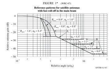
$G_{max} = 44.45 - 10 \log (\varphi_{01} \cdot \varphi_{02}) \qquad \text{dBi} \quad (\text{WRC-07})$ Curve A: dB relative to main beam gain  $-12 (\varphi/\varphi_0)^2 \qquad \qquad \text{for } 0 \le (\varphi/\varphi_0) \le 0.5$
