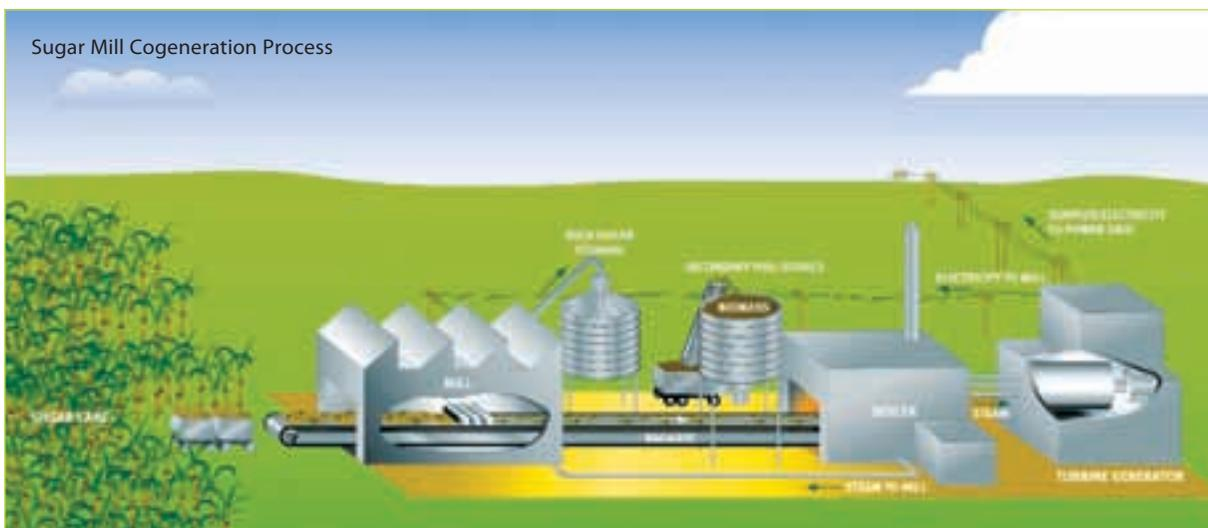
**Figure 6 – Sugar Mill Cogeneration Process.** Courtesy Rocky Point Sugar Mill
