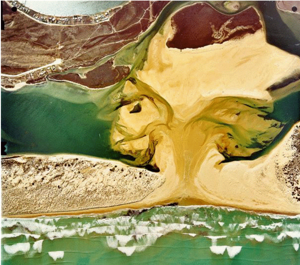
Figure 2.2 River Murray Mouth in April 1981 showing full blockage at the Mouth and restriction of water exchange between the Goolwa (left) and Tauwitchere (right) Channels.
