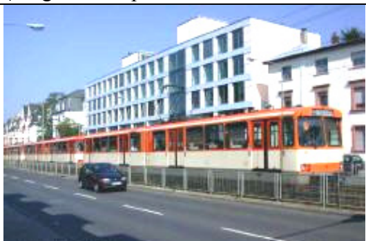
↑ Light rail on dedicated tracks in center of 2x2 lane major road; high flexibility; from 70 off peak to 400 passengers depending on length of train (up to 100 m); 1 driver
