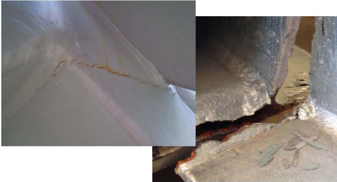
Figure 4.2: Steel cracking on imported fabricated product 49
