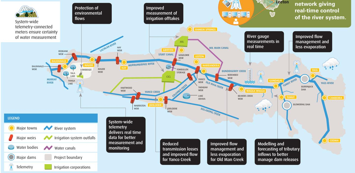
The Murrumbidgee Computer Aided River Management (CARM) project is an upgrade of infrastructure and installation of new interactive river flow management technology throughout the river system, making control and measurement of water flows much more precise and responsive, delivering water at the right quantity, time and place.
