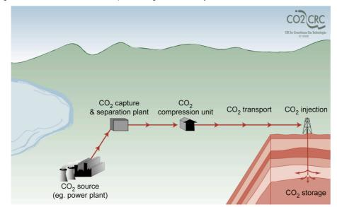
The diagram below illustrates a conceptual integrated CCS system.
