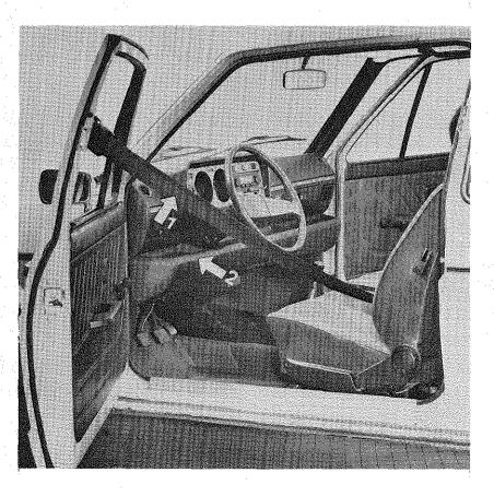
The belt is secured by an inertia retractor to the front seat and the other end is anchored to the door pillar. When the door is closed the belt is automatically applied over the chest (as illustrated - arrow 1). In place of a lap belt there is an energy-absorbing knee bolster (arrow 2) which prevents the passenger from slipping out under the belt in a collision. The absence of a lap belt obviously reduces the effectiveness of the device in side collisions.
