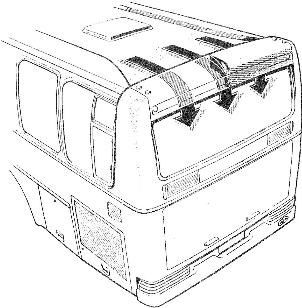
Figure 3: Air deflectors reduce the amount of dirt accumulation on the rear of a bus
