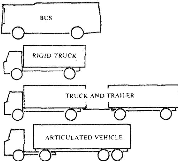
Figure 2: Vehicle types currently allowed to operate under general permits in certain parts of Australia
