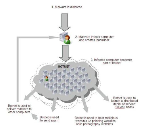
Figure 2.1 Initiation, growth and function of a botnet
