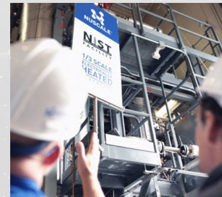
One-third scale NIST-1 Test Facility
