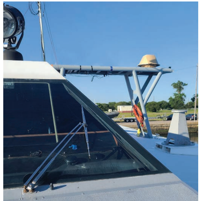
Photo caption DroneShield DroneSentry-X ship mounted direction-finding UAS sensor (using RF technology).
