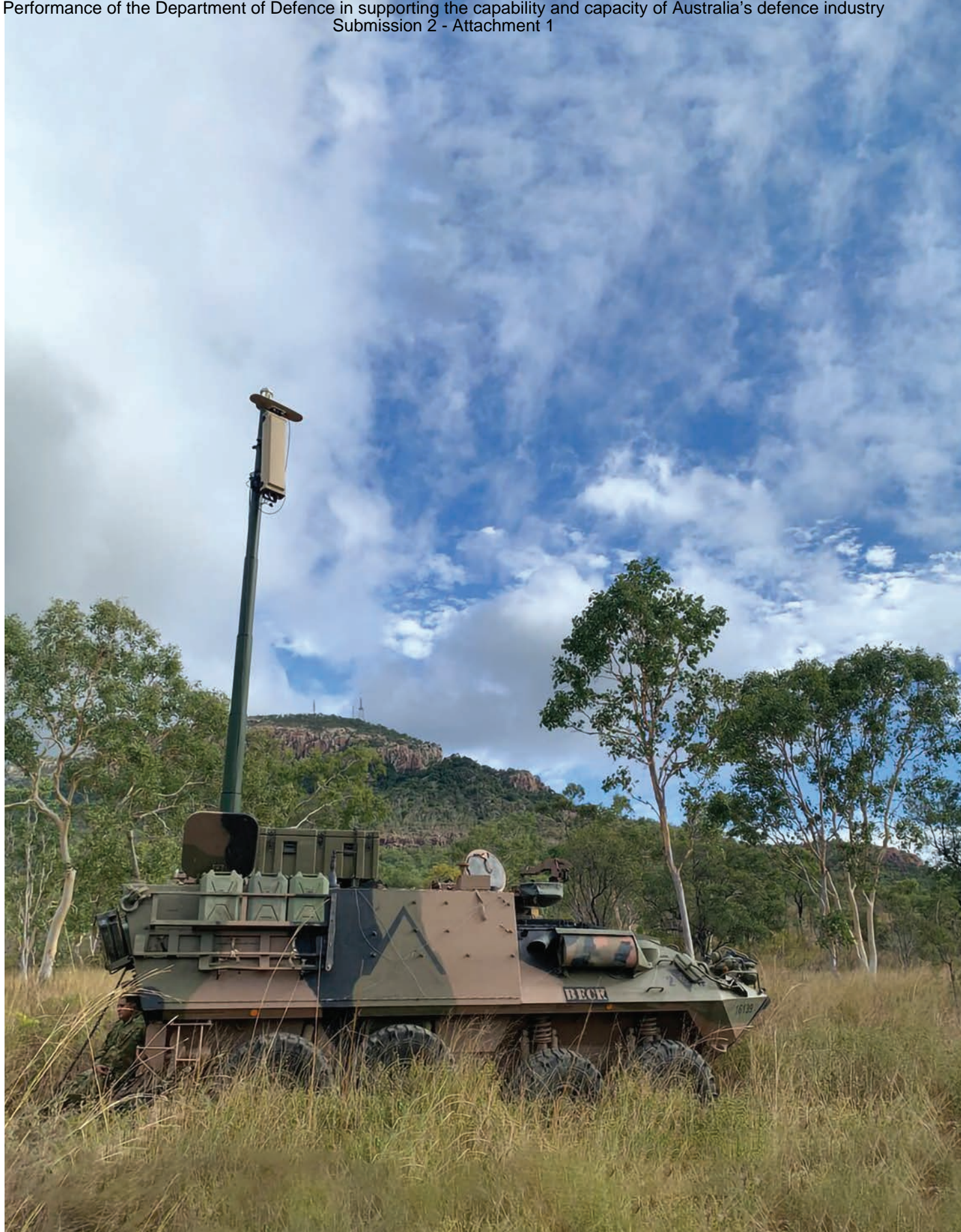
Photo caption DroneShield RfOne passive far-range drone detection sensors on an Australian Light Armoured Vehicle.
