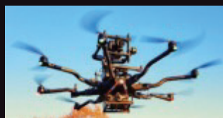
Figure caption: Sample of group 1 UAS capable of heavier payload modification. Higher-end group 1 UAS are modifiable for a range of payloads, including surveillance and explosive material.
