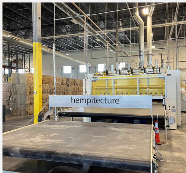
Image: Final stage of production for hemp insulation batts
