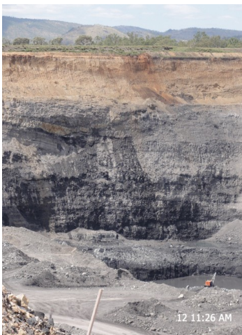
Sonoma Coal Mine pit (Strip 8/9, Block 10) 12.9.10 11.26am. Dewatering Pump running at approx. 50 litres/sec
