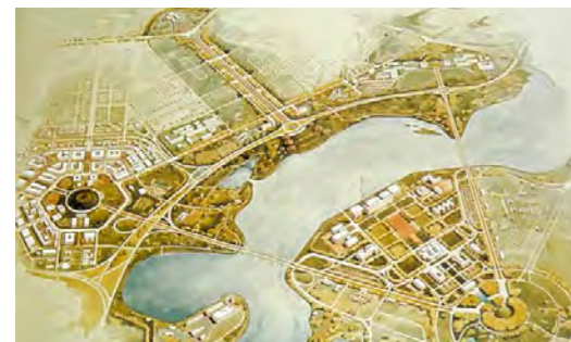
Figure 65: Holford's scheme, as shown on an NDCD plan, showing a curved Parkes Way, less geometric northern edge to Central Basin, splayed edges to the south and park like landscaping.
