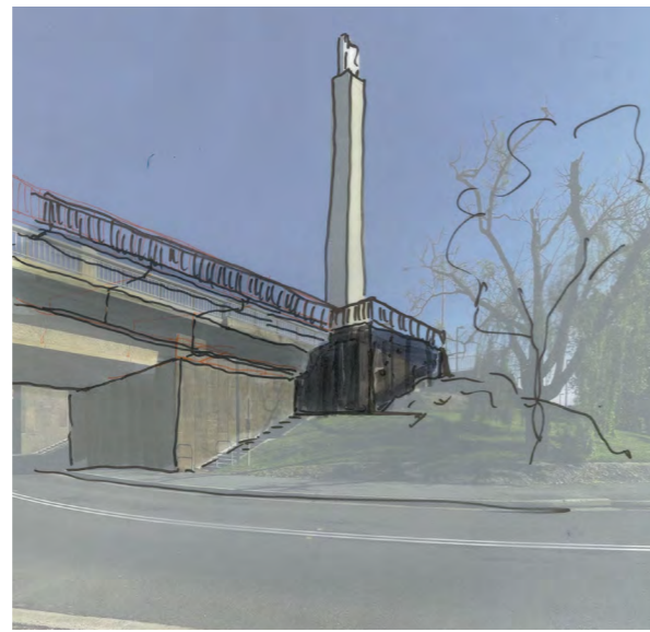
Abutment is extended on three sides around Pylon, to be faced in brown granite as per existing. Original appears to be Tarana granite - quarry now closed. Close approximation is Desert Rose from UrbanStone.
