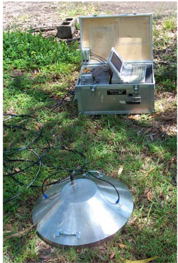
Fig. 3 Radon and thoron emanometer and field laptop (Lawrence 2005)
