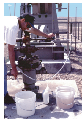
Figure 2. USGS chemist prepares to sample water from the wellhead of a coalbed methane well. Wellhead sampling and on-site sample preservation and analysis are critical to obtaining good quality compositional and isotopic data. Many parameters, such as pH, alkalinity, and trace-metal content, change rapidly once the water is removed from the well.
