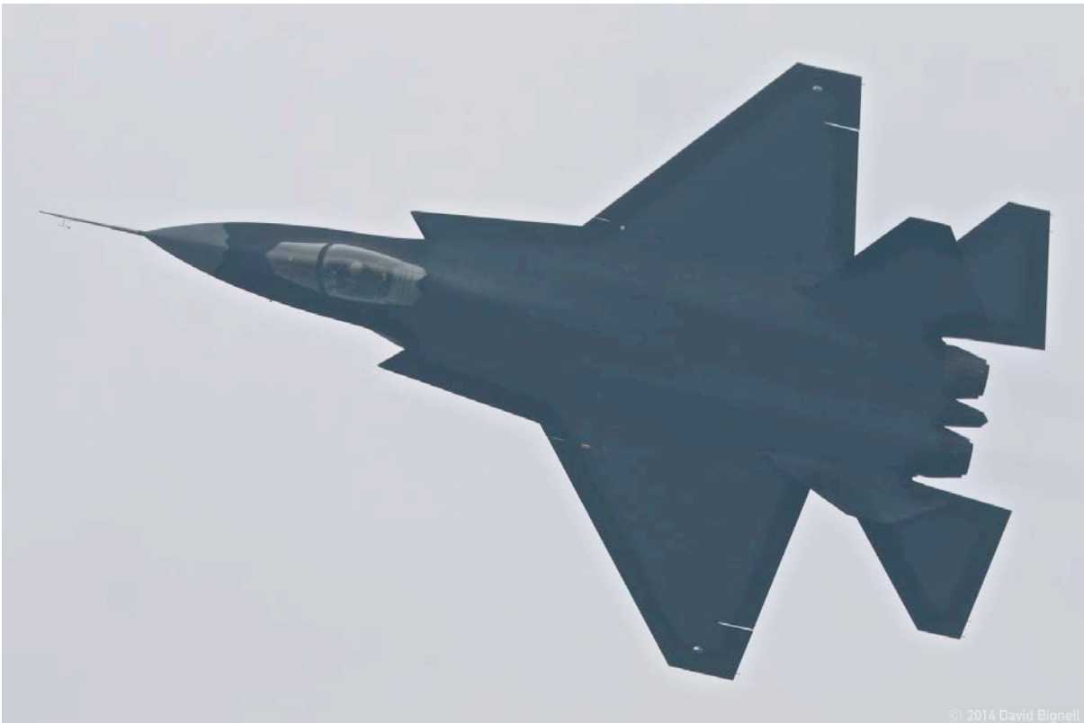
Above, below: Shenyang J-31 prototype at the 2014 Zhuhai air show. This Chinese stealth fighter is commonly described by Western media as a copy of the F-35, but key stealth and aerodynamic features appear to be borrowed from the F-22A Raptor (David Bignell via APA).
