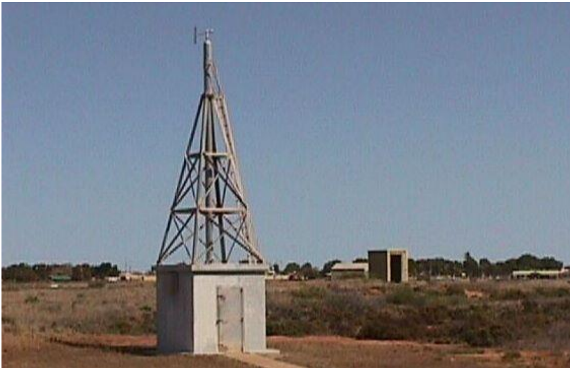
Figure 2.2.6 Dines anemometer at Carnarvon, WA (photo from BoM website http://www.bom.gov.au/weather/wa/carnarvon/photos.shtml )
