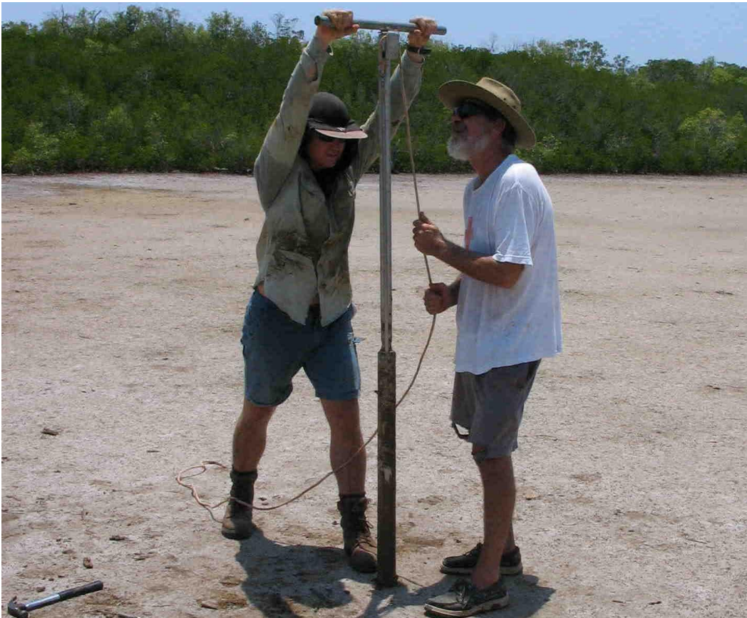
Figure M.4 Coring with piston sampler.
