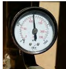
Photo taken at 4 th monthly inspection 5.5.17 – 800kpa pressure in fire system on arrival
