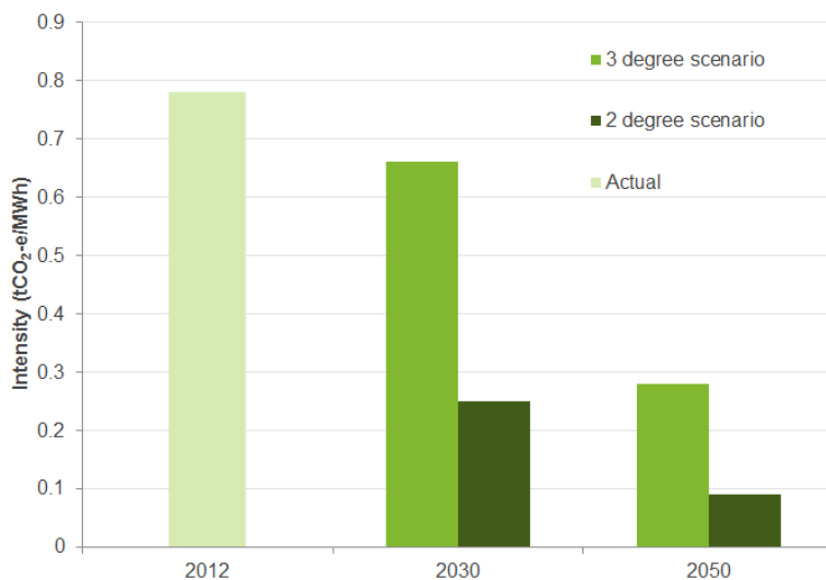
FIGURE 5: CHANGES IN EMISSIONS INTENSITY OF AUSTRALIA'S ELECTRICITY SUPPLY TO 2050 2 AND 3 DEGREE SCENARIOS
