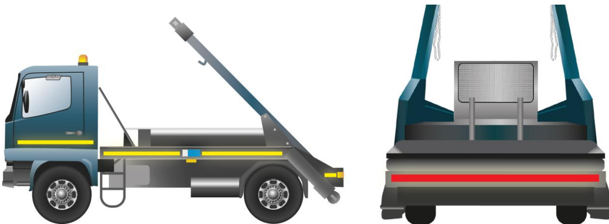
Figure 16: Skip loader with line markings 6
