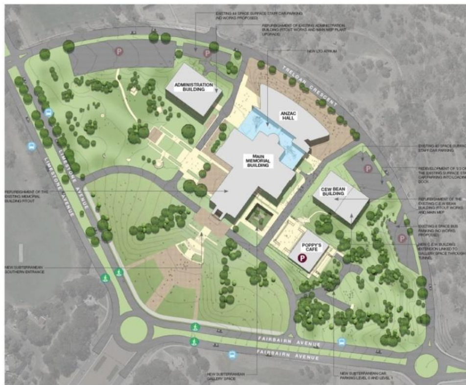
Figure 3-2 – Option 2 Additional gallery space underground to the east (the only above ground change is the Glazed Link between the Main Building and Anzac Hall)
