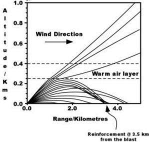
Atmospheric conditions can, on occasions, concentrate or focus air vibration in certain directions and distances from the blast. Weather conditions that include an 'inversion' or a layer of warm air between colder air layers, such as exists on smog pollution days, can cause an increase of up to 10 or more decibels at distances from 2-5 km from the blast. The reinforcing mechanism is demonstrated on the left.
