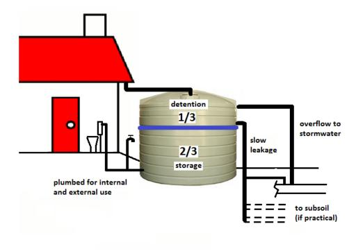
Figure – Detention Enabled Stormwater Tanks
