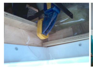
Figure 22: Blower door apparatus modified for testing roof cavity,
