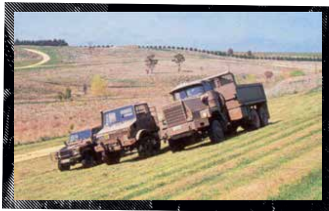
Test driving on 30degree incline
