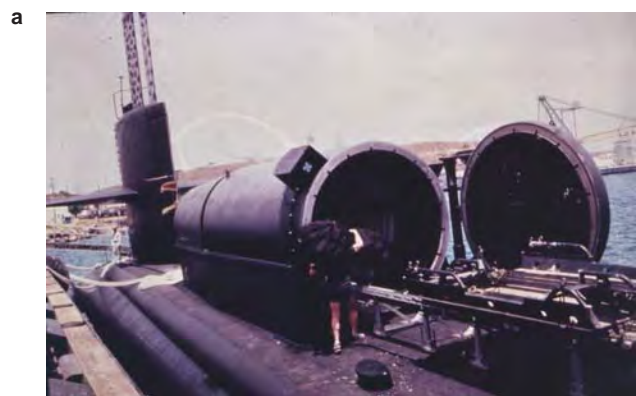
Fig. 37-12. (a) A Dry Deck Shelter (DDS) is being installed onto a host submarine. (b) US Navy SEAL (sea, air, land) divers launch a SEAL delivery vehicle (SDV) from the DDS. Photographs: Courtesy of US Special Operations Command, MacDill Air Force Base, Tampa, Fla.
