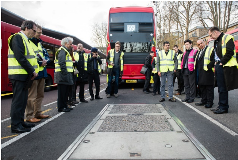
Figure 50: London Buses Inductive Charging (Source: 164 )
