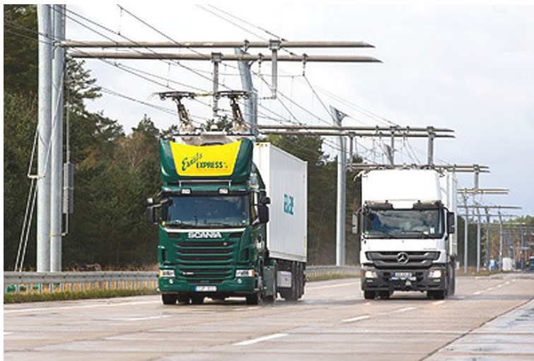
Figure 55: Overhead Powered HGVs (Source: ETA.co.uk)
