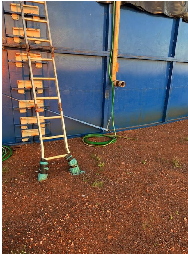
8 Hydrera potential siphoning set up of highly contaminated fracking flowback water with ladder in place
