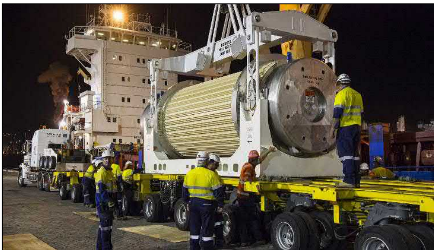
Figure 74 TN81 Container being transported (Department of Industry, Innovation and Science, 2016)
