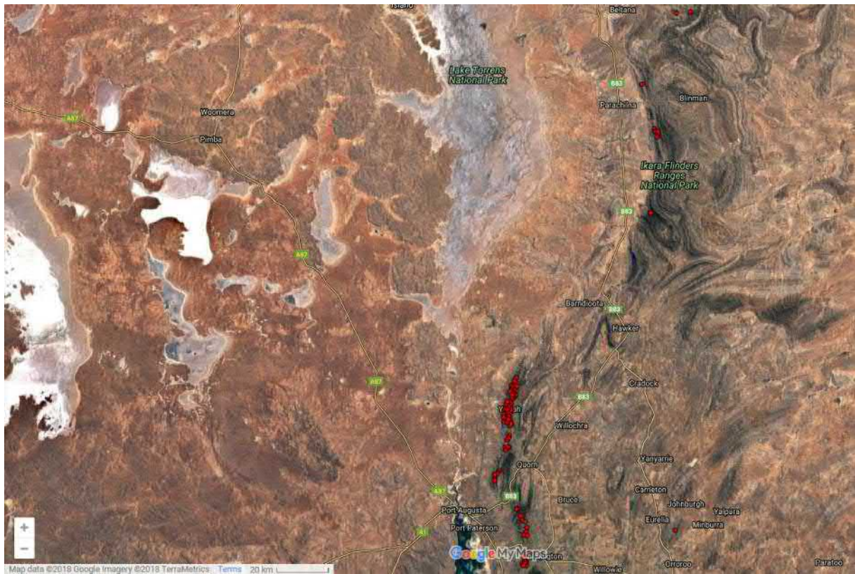
Figure 87 Pumped Hydro atlas, red circles indicate identified potential pumped hydro sites [29]
