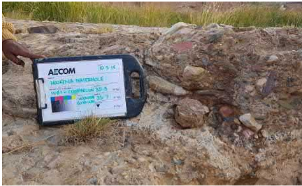
Comparison of sonic core sample from W01 (35.5 - 35.7 m bgs) with Hookina Waterhole outcrop – 10/05/18
