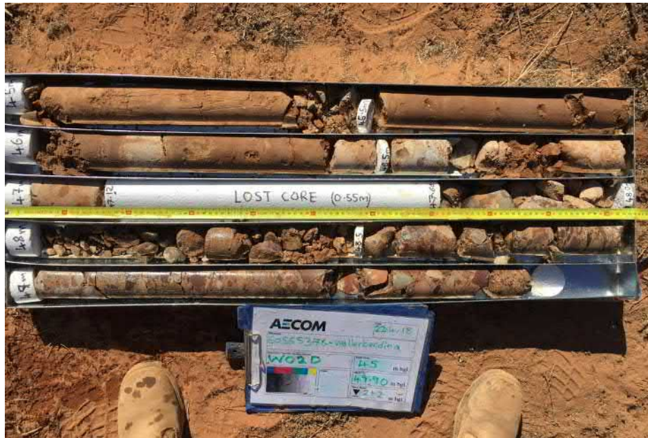
Figure 33 Core box showing intersected conglomerate at W02D
