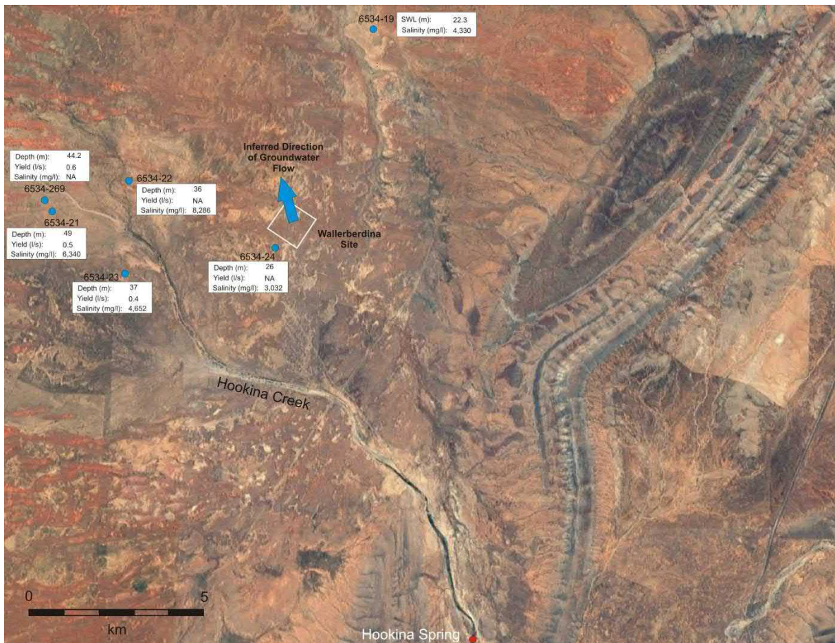
Figure 36 WaterConnect registered bore information and inferred watertable aquifer flow direction (23/05/18)
