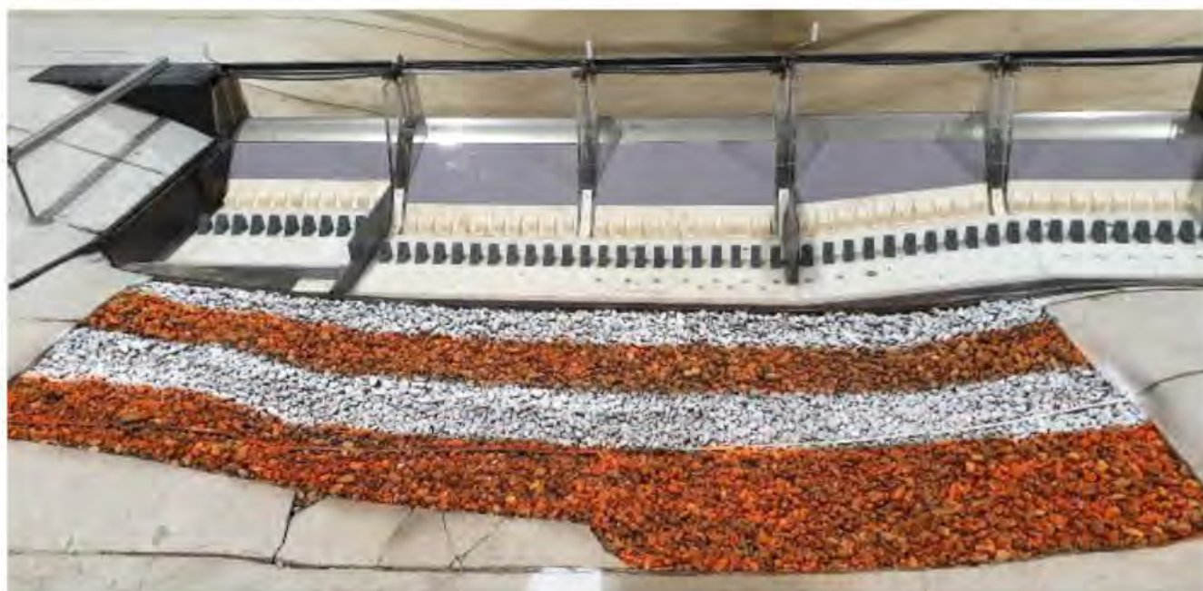
Figure 16 Removable bed scour test, prior to run (note spray-painted gravels)
