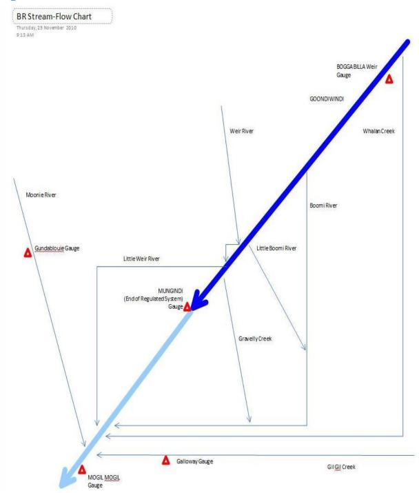
As shown in Fig 1, the effluent streams Whalan Creek, Boomi River, Little Boomi River and Gravelly Creek all re-join the main river (Barwon River) above the Mogil Mogil gauge, as does the Gil Gil Creek. The Moonie River also joins above Mogil Mogil, but the gauge at Gundablouie can be used to subtract that figure from this example
