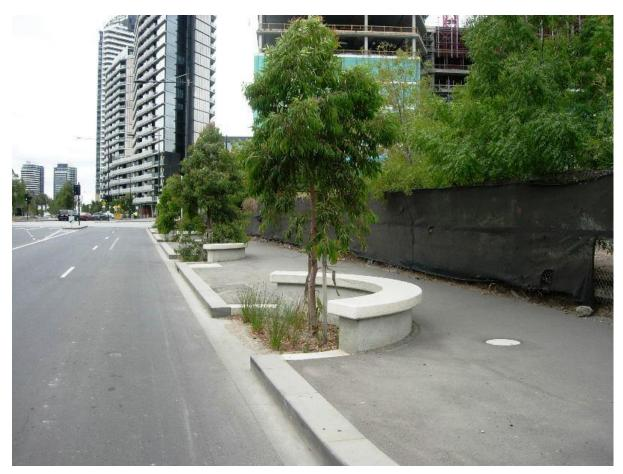
Figure 42: Batman Drive bioretention tree pits, Docklands Melbourne. By author.
