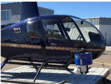
Figure 3-5 Helicopter deployment of the multispectral turret shown in Figure 3-1
