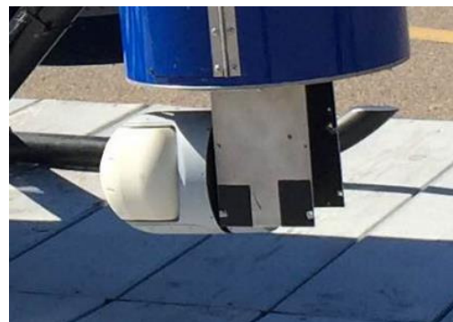
Figure 3-5 Helicopter deployment of the multispectral turret shown in Figure 3-1
