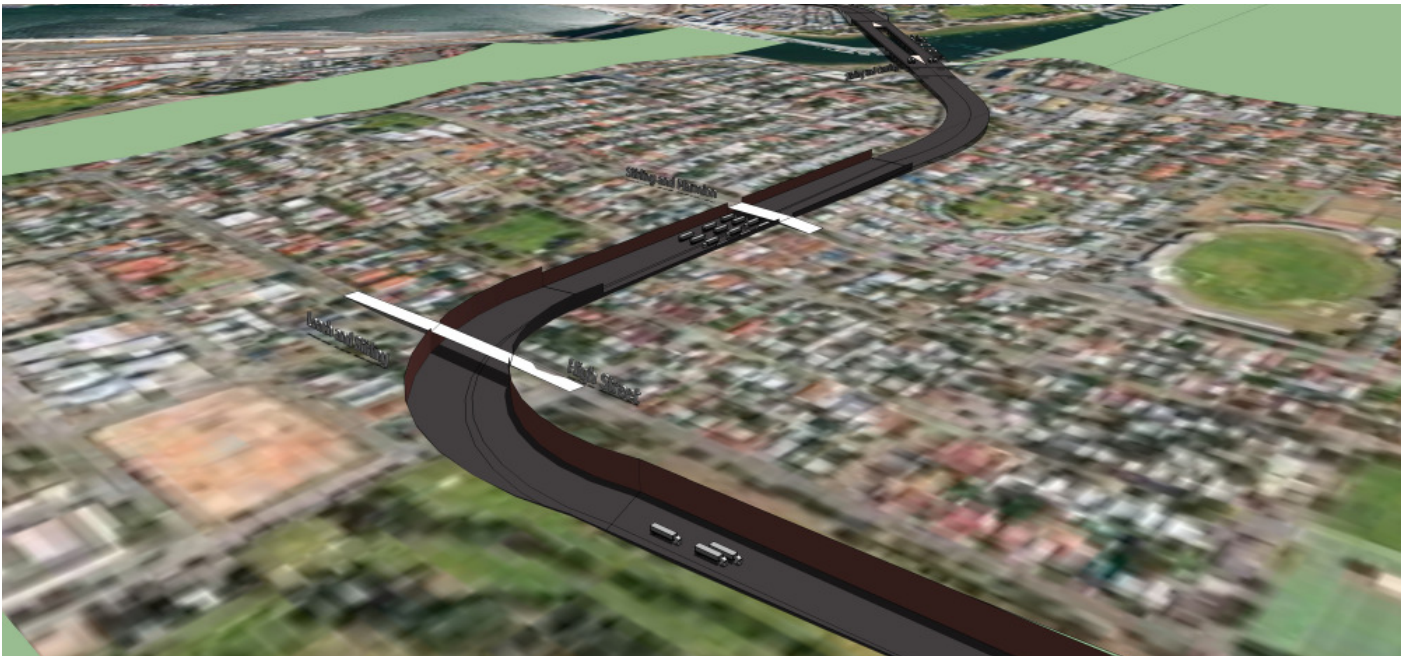
Figure 13. The new proposal for the High/Leach and Stirling intersection. Leach is lowered into an open trench to slide under Carrington, High and Marmion Street.
