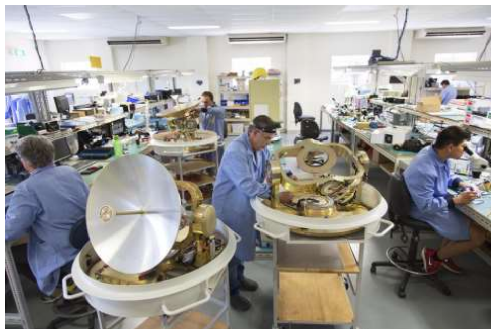
Figure 1. These figures show an example of the satellite communications on-the-move terminals designed and manufactured in Australia by EM Solutions. Similar terminals are in use in Japan, and in early July successfully passed qualification testing in Ottawa, Canada for a CDF tender demonstration. EM Solutions was unable to tender these to the ADF because the relevant procurement tender (JP2072) was bulked up to such an extent that only multinational bidders had the capability to respond. EM Solutions was a subcontractor to one prime contractor that chose, in the end, to propose a US-based solution that was viewed as more field-ready and less risky.
