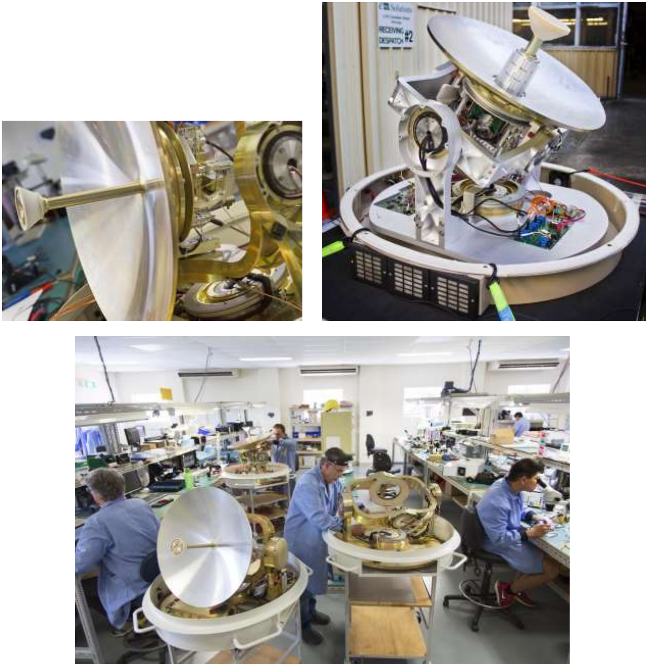
Figure 1. These figures show an example of the satellite communications on-the-move terminals designed and manufactured in Australia by EM Solutions. Similar terminals are in use in Japan, and in early July successfully passed qualification testing in Ottawa, Canada for a CDF tender demonstration. EM Solutions was unable to tender these to the ADF because the relevant procurement tender (JP2072) was bulked up to such an extent that only multinational bidders had the capability to respond. EM Solutions was a subcontractor to one prime contractor that chose, in the end, to propose a US-based solution that was viewed as more field-ready and less risky.
