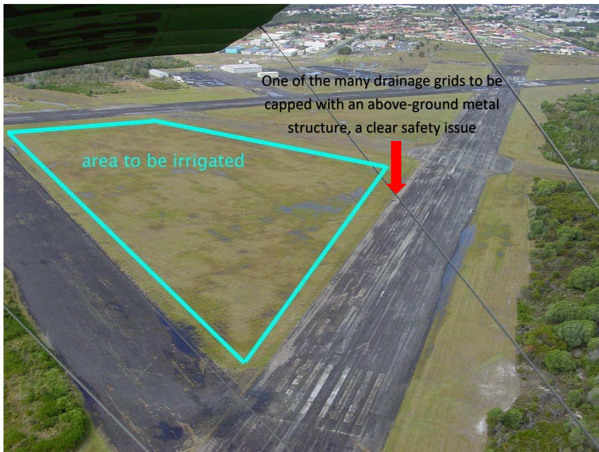
Figure 3: Area to be irrigated with effluent located within the area bounded by the four runways of the airfield. There are many drains within the area which council planned to cap with above-ground metal covers, a clear risk for collision in the event of aircraft runoff. The irrigation system would have cut through the whole of the underground drainage system for rainwater leading to flooding of the aerodrome during heavy rain, a not uncommon occurrence for which the drainage system was built in WWII.
