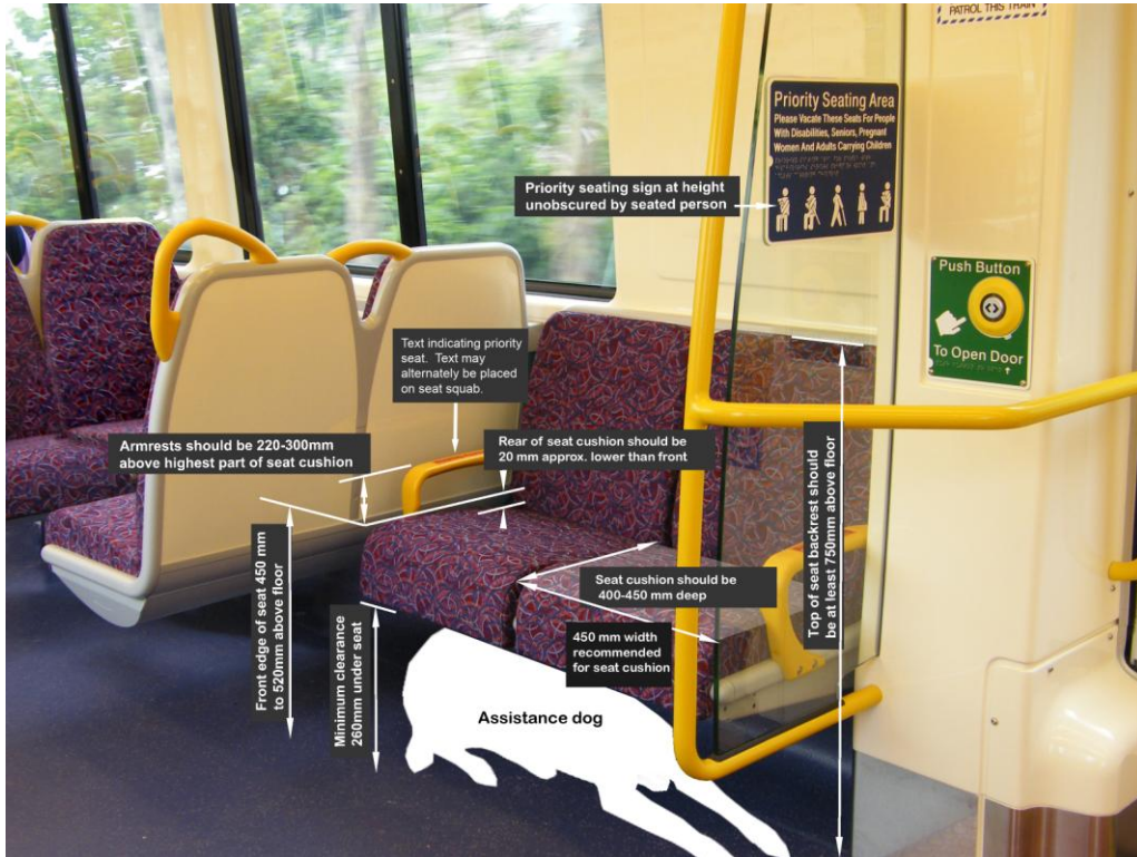
Figure 7.2.1.c. Examples of priority seating dimensions and specifications (dimensions in millimetres). Note: Sign text may be sentence or title case.
