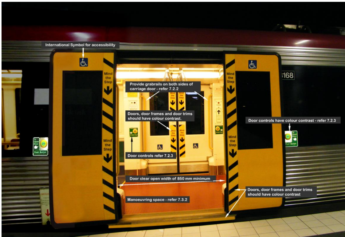
Figure 7.1.1.a. Examples of carriage entrance and door specifications (dimensions in millimetres). Note: Sign text may be sentence or title case.
