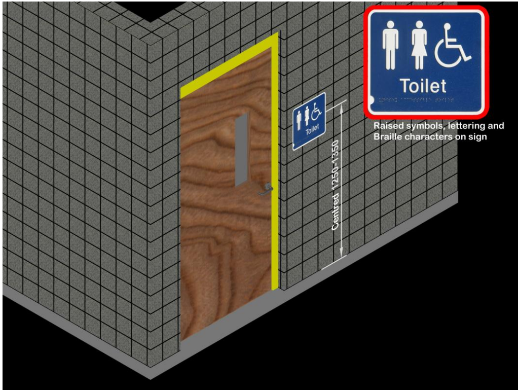
Figure 5.3.2. Example of a tactile and Braille sign at toilet door (dimensions in millimetres).
